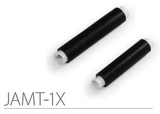
Cold shrink joint kit for MV single-core cables up to 36 kV with extruded insulation
