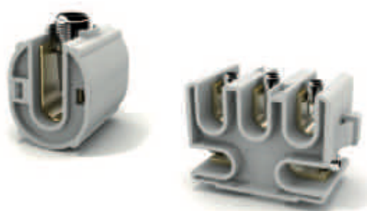
Pre-assembled terminal blocks provided with Shark® 600 Series joints have brass contacts with screw-type clamping and PA 6.6 insulating body self-extinguishing of class V2
